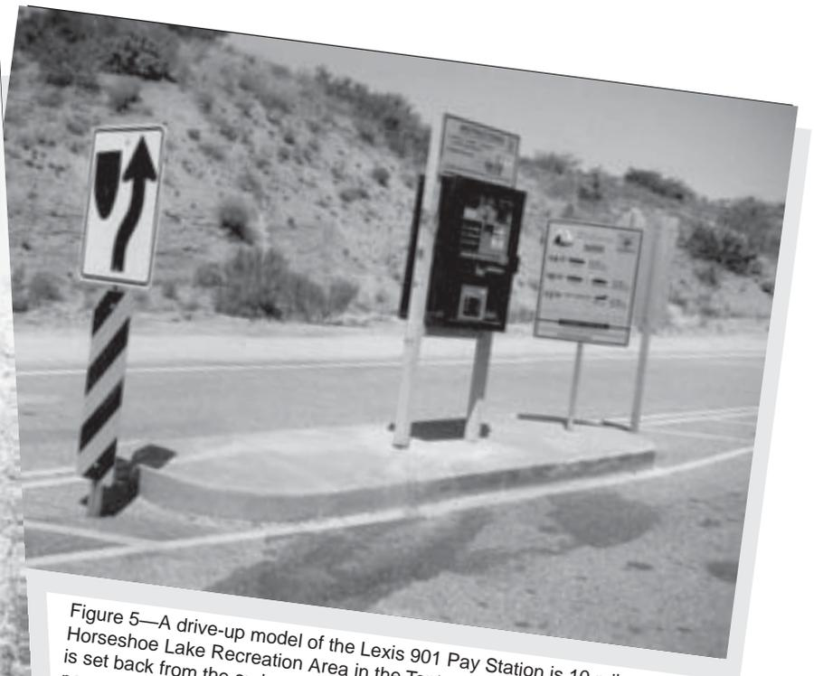
Figure 5—A drive-up model of the Lexis 901 Pay Station is 10 miles from the Horseshoe Lake Recreation Area in the Tonto National Forest. This machine is set back from the curb, forcing motorists to step outside their vehicles to pay the fee.
