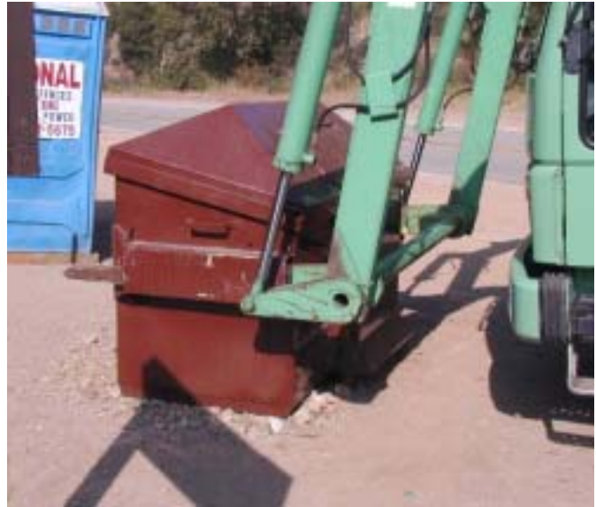
Figure 3—A frontloader refuse collection truck emptying a dumpster.
