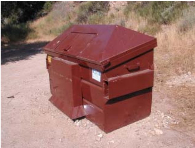
Figure 1—Two-cubic-yard bearproof dumpster with access panel and sloped lid.
