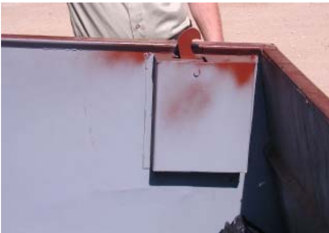
Figure 2—The self-locking gravity latch mechanism.
