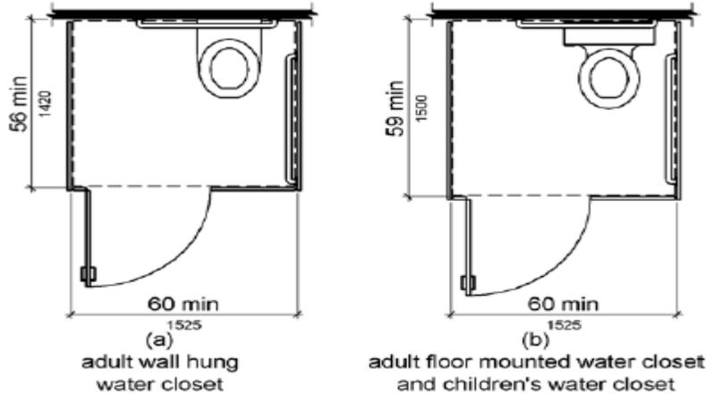
Figure 604.8.1.1 Size of Wheelchair Accessible Toilet Compartment
