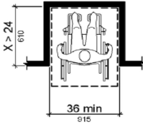
Figure 305.7.1 Maneuvering Clearance in an Alcove, Forward Approach
