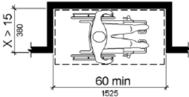
Figure 305.7.2 Maneuvering Clearance in an Alcove, Parallel Approach
