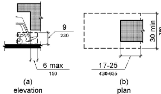
Figure 306.2 Toe Clearance
