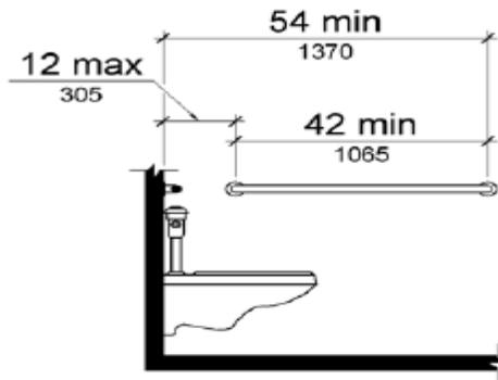
Figure 604.5.1 Side Wall Grab Bar at Water Closets
