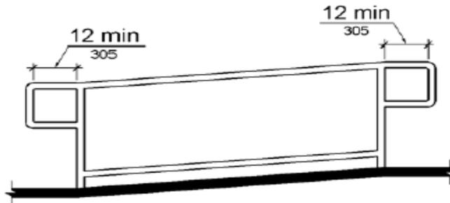
Figure 505.10.1 Top and Bottom Handrail Extension at Ramps
