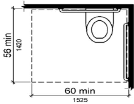
Figure 604.3.1 Size of Clearance at Water Closets
