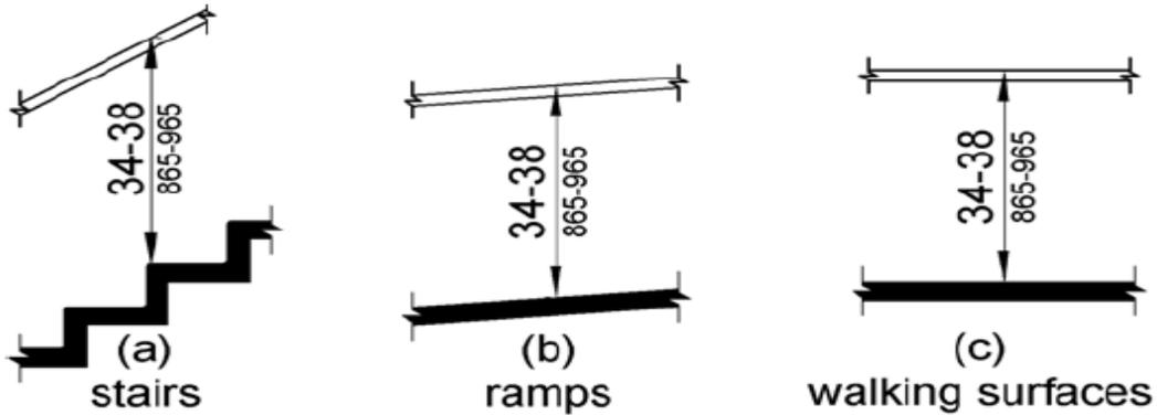
Figure 505.4 Handrail Height
