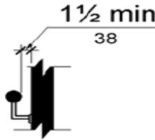
Figure 505.5 Handrail Clearance
