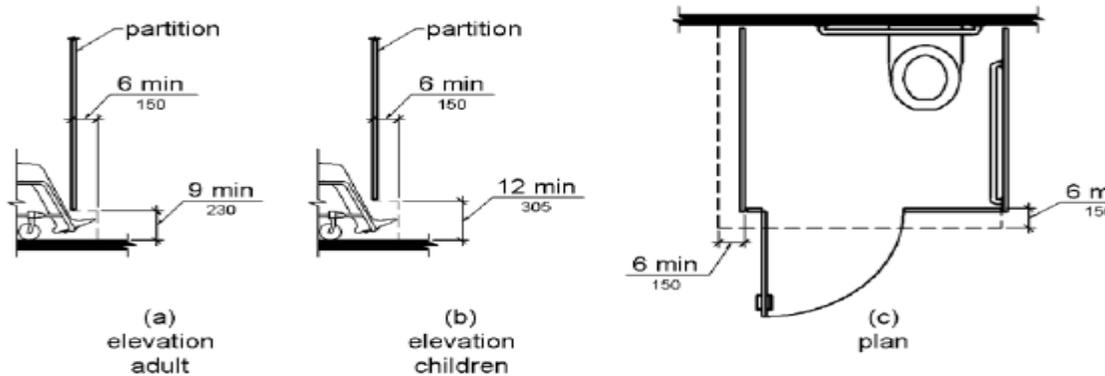
Figure 604.8.1.4 Wheelchair Accessible Toilet Compartment Toe Clearance
